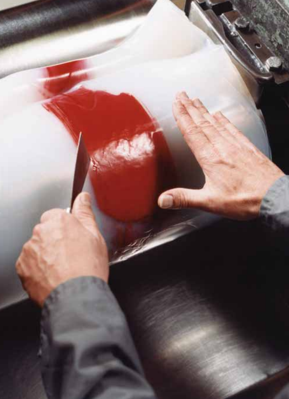
ELASTOSIL® COLOR PASTES blend especially easily and fast into rubber compounds on the roll mill
